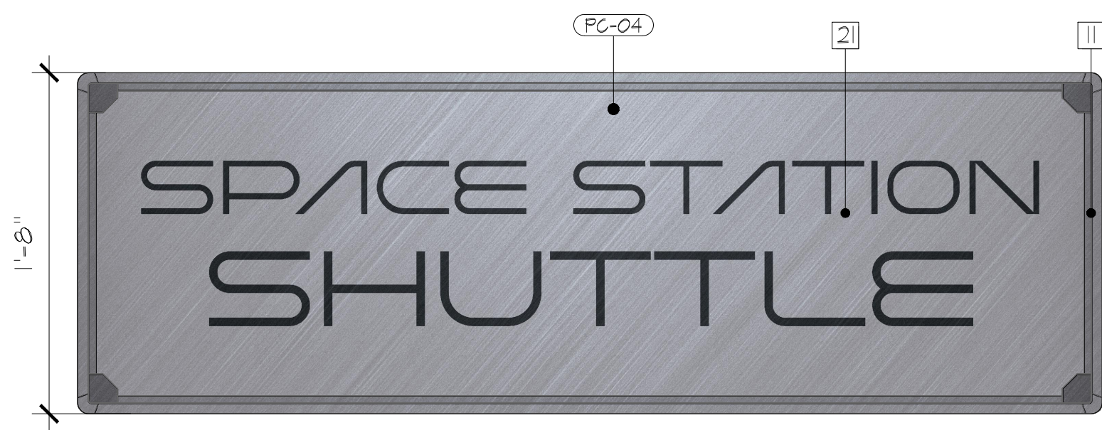
GR.03.002 - SPACE STATION MOUNTED SIGN - DETAIL SCALE: 1 1/2" = 1' D-625
