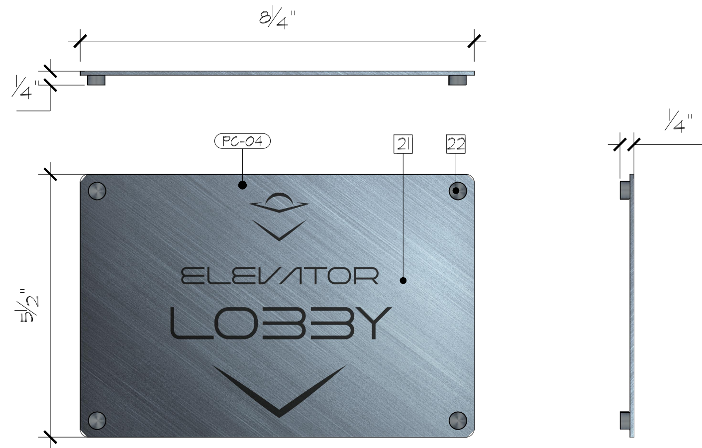
GR.01.004 - SPACE STATION MOUNTED SIGN - DETAIL SCALE: 6" = 1" D-623
