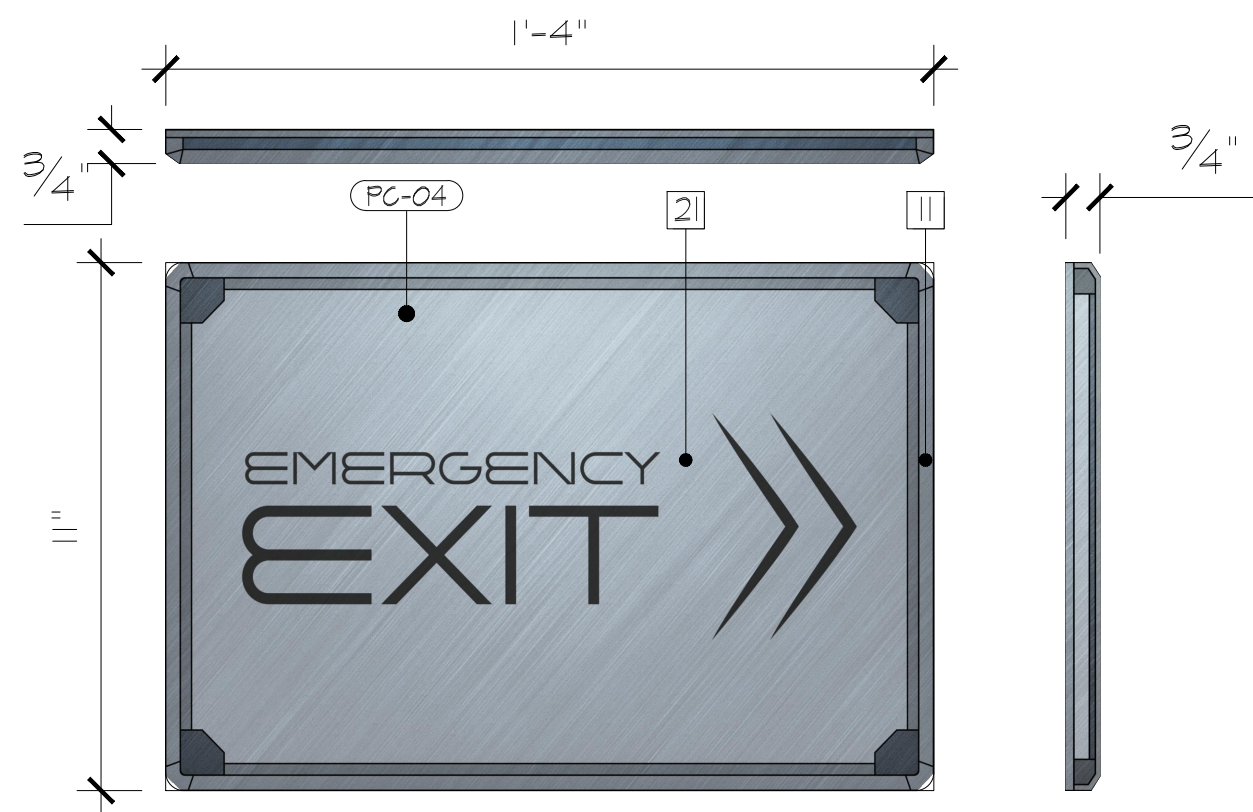
GR.03.001 - SPACE STATION OPERATIONS SIGN - DETAIL SCALE: 3" = 1' D-624
